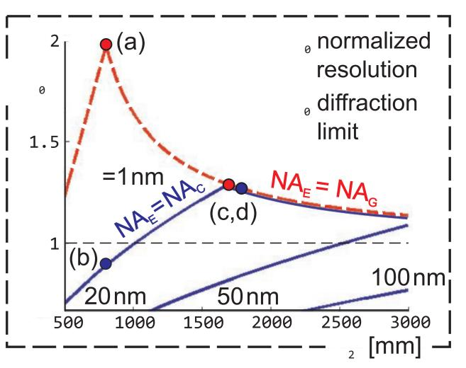
Figure 9: The normalized image resolution in dependence on the CCD position \_\_\_\_\_ for the Q-M light (dashed line) and the broadband light (solid
