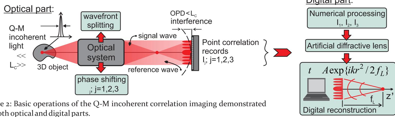
Figure 2: Basic operations of the Q-M incoherent correlation imaging demonstrated for both optical and digital parts.
