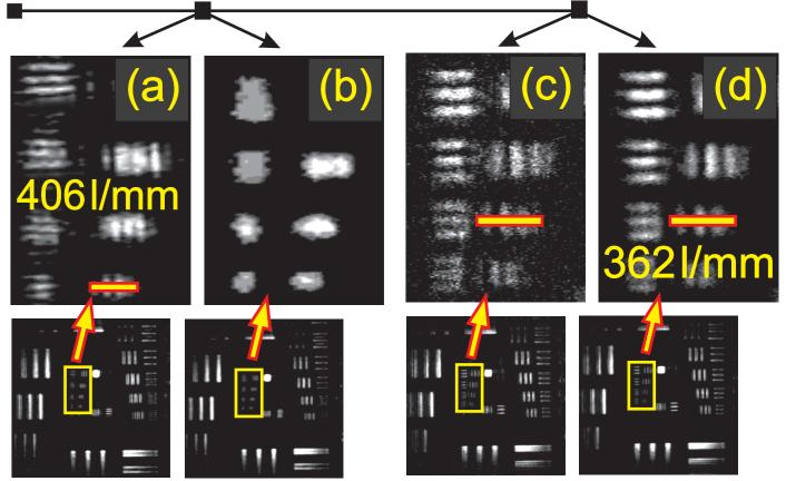
Figure 11: Reconstruction of the USAF target in the positions (a)-(d) in Fig. 9. Resolution obtained for =1nm and 20 nm is significantly different in the positions (a) and (b) but remains unchanged in the positions (c) and (d).
